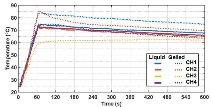
**Figure 7:** Payload temperature evolution comparison for 200g of deionized water in their liquid and gelled (4g Agar-Agar per liter of DI-water) versions at 4 measurement points during its continuous microwave irradiation (800W rated power) for 1 minute, and posterior resting while cooling down.
