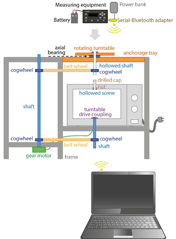
Figure 1: Schematic of the rotating monitoring setup.
