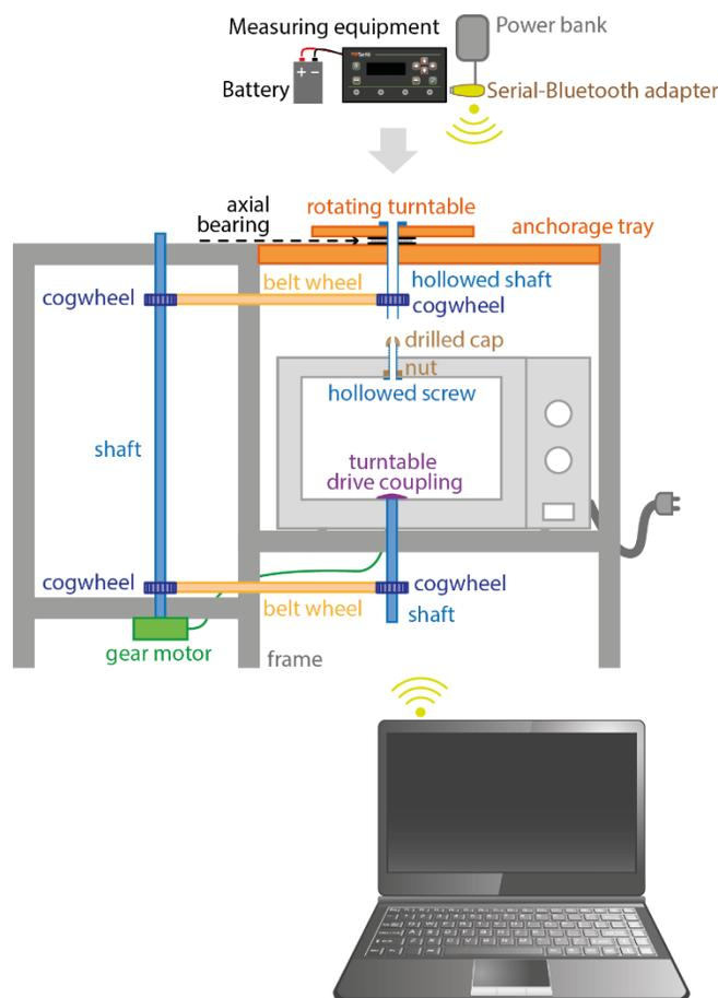
**Figure 1:** Schematic of the rotating monitoring setup.
