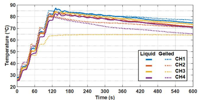
**Figure 8:** Payload temperature evolution comparison for 200 g of deionized water in their liquid and gelled (4 g Agar-Agar per liter of DI-water) versions at 4 measurement points during its pulsed microwave irradiation (450 W rated power) for 2 minutes, and posterior resting while cooling down.
