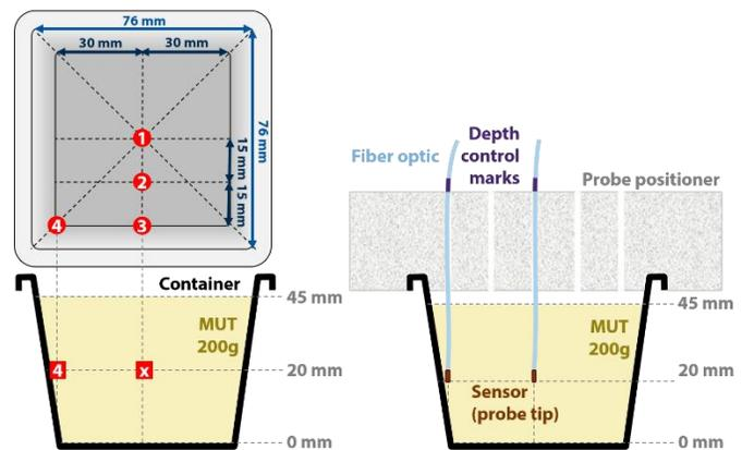
**Figure 4:** Probe positioner and measuring point locations.
