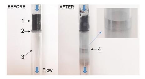
**Figure 8.** Reference sample before and after microwave treatment. (1) sample, (2) quartz frit to support the sample, (3) quartz holder, (4) volatilized zinc from the sample deposited on the quartz holder walls after treatment.
