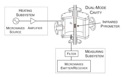
**Figure 1.** Schematic view of experimental set-up with the microwave dual system for heating and measuring the dielectric properties of samples during the carbothermic reduction process. The sample is placed inside a quartz holder and located in the center of the cylindrical microwave cavity.
