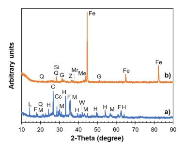
**Figure 7.** X-ray diffraction (XRD) pattern of reference sample (C/O = 100%) (**a**) before—see Table 2—and (**b**) after microwave treatment. Q = Quartz, Si = Silicon, Cc = Calcite, G = Gehlenite, Z = Zincite, Mr = Merwinite, Me = Melilite, Fe = Iron, L = Lepidocrocite, F = Franklinite, M = Magnetite, H = Hematite, C = Carbon (graphite), W = Wüstite.
