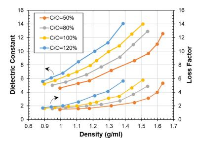
Figure 6. Dielectric properties of samples with different carbon content as a function of density.
