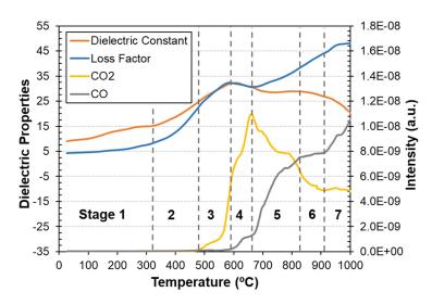
**Figure 3.** Dielectric properties and mass spectrometry (CO and CO<sub>2</sub> gases) of reference sample (C/O = 100%) as a function of temperature.
