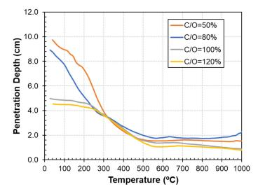
Figure 5. Penetration depth of samples with different carbon content as a function of temperature.
